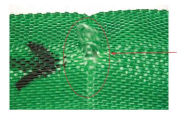
THE DAMAGE: Holes/Snags/Pulls exposing internal core yarns.
